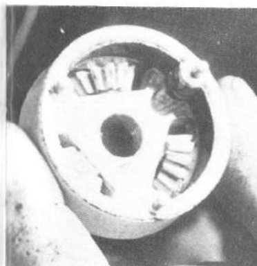
Below right: Various parts of the clutch and brake assembly.
